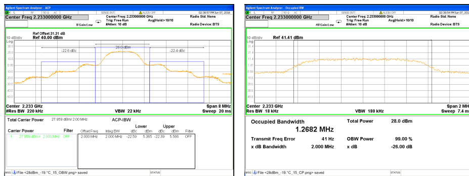
Figure 6 Spectrum spread of 28 dBm output at −20 °C: Adjacent Channel Power (left) and Occupied Bandwidth (right).
