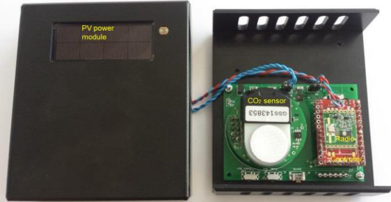
Fig. 4: The developed 70 × 50 × 20 mm autonomous IoT node for building ventilation: on the left image the window area is the mounted PV energy harvesting power supply, while on the right image the sensor mounted can be seen on the left hand-side, and the microcontroller (red board) on the right. The green radio board sits on top of the microcontroller
