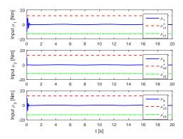
Fig. 3. Control input  $\mu$  under model-based control (23).
