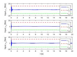
Fig. 10. Control input  $\mu$  under output-feedback-based adaptive neural control (43)
