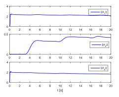
Fig. 7. Euclidean norm  $\|\hat{\theta}_i\|$ , i=1,2,3 under state-feedback-based adaptive neural control (30).
