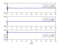
Fig. 2. Tracking error  $z_1 = x_1 - x_d$  under model-based control (23).
