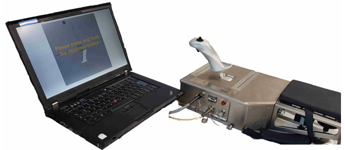
Fig. 12: Experimental setup in the first user study. The DLR force feedback joystick can be seen on the right, and the laptop simulating the VE on the left.
