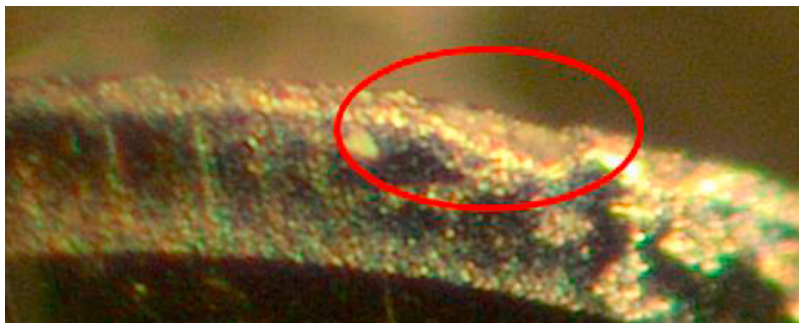
Figure 9: Chipping on tool edge of carbide C
