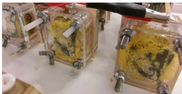
Figure 2. A triplicate of test MFCs with cathode electrodes heavily colonised with yellow P. polycephalum .
