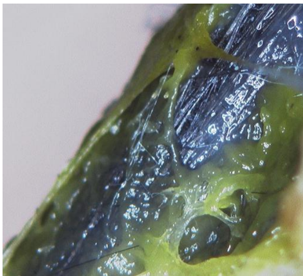
Figure 6. P. polycephalum colonising the cathode electrode (50x magnification, Hirox Europe Ltd, Limonest, France). The carbon veil electrode appears glossy and wet due to the presence of mucosa generated by P. polycephalum .
