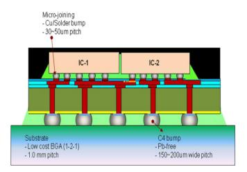
FIG. 22. Schematic of a typical 2.5D TSI system with two-die side-by-side integration.
