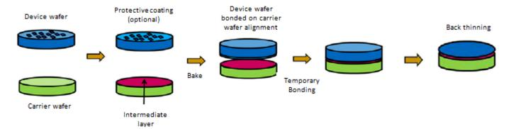
FIG. 30. A typical temporary bonding process flow.
