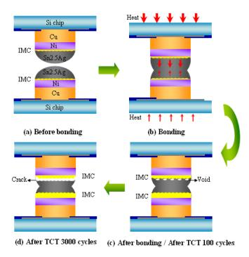
FIG. 26. Schematic diagrams of the failure mechanism of micro-joint. (a) Before bonding, (b) bonding, (c) after bonding/after TCT 100 cycles, and (d) after TCT 3000 cycles.
