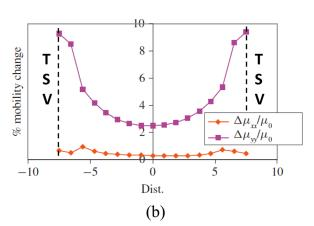
FIG. 84. Percent change in mobility due to the presence of  $10 \,\mu m$  TSVs which are  $25 \,\mu m$  apart for (a) p-MOSFET and (b) n-MOSFET. TSVs align with [110]. Packag., Manuf. Technol. 1(9), 1328 (2011). Copyright 2011 Institute of Electrical and Electronics Engineers.
