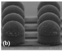
FIG. 23. Cu pillar bumps (a) with severe Cu post undercut and (b) fabricated with optimized process having minimized Cu post undercut.
