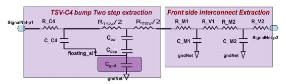
FIG. 92. Line extraction model in 2.5D TSI extracted using 2 step extraction methodology.
