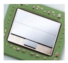
FIG. 3. Xilinx Virtex 7HT with a 2 slices of FPGA integrated with SERDES IC. 12 Reproduced with permission from Madden *et al.*, "Advancing high performance heterogeneous integration through die stacking," in Proceedings of European Solid-State Device Research Conference (ESSDERC) (2012). Copyright 2012 Institute of Electrical and Electronics Engineers.
