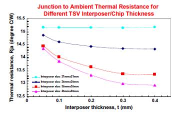
FIG. 62. Junction to ambient thermal resistance for different TSV interposer thickness. <sup>109</sup> Reproduced with permission from Hoe *et al.*, "Effect of TSV interposer on the thermal performance of FCBGA package," in 11th IEEE Electronics Packaging Technology Conference (EPTC) (2009). Copyright 2009 Institute of Electrical and Electronics Engineers.
