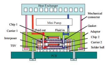
FIG. 72. Scheme of the integrated liquid cooling system for 3D stacked module (no to the scale). Reproduced with permission from Khan *et al.*, "3-D packaging with through-silicon via (TSV) for electrical and fluidic interconnections," IEEE Trans. Compon., Packag., Manuf. Technol. 3(2), 221 (2013). Copyright 2013 Institute of Electrical and Electronics Engineers.
