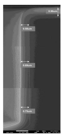
FIG. 13. SEM images of O3-TEOS liner oxide for a TSV with the diameter of 10  $\mu m$  and depth of 100  $\mu m$ .
