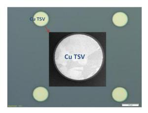
FIG. 17. Optical inspection and SEM inspection (inset) results of  $10~\mu m \times 100~\mu m$  TSV after CMP process.
