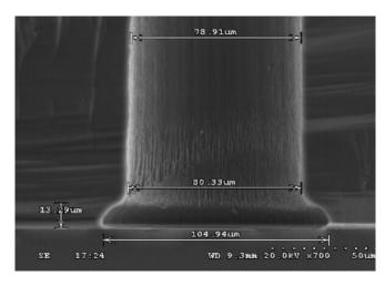
FIG. 12. Notching observed at the interface between Si and SiO<sub>2</sub> layer.<sup>27</sup>
