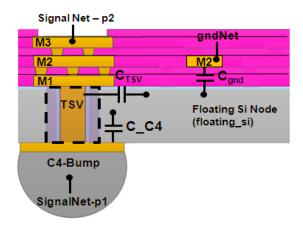
FIG. 91. Parasitic capacitances associated with TSV, C4 bump and ground net in 2.5D TSI.
