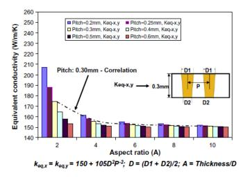
FIG. 54. Equivalent thermal conductivity in normal x,y-direction (keq,x) and (keq,y). <sup>109</sup> Reproduced with permission from Hoe *et al.*, "Effect of TSV interposer on the thermal performance of FCBGA package," in 11th IEEE Electronics Packaging Technology Conference (EPTC) (2009). Copyright 2009 Institute of Electrical and Electronics Engineers.
