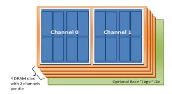
FIG. 102. Schematic diagram of an 8-channel high bandwidth memory. 14
