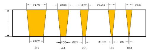
FIG. 52. TSV geometry for different aspect ratios. 109 Reproduced with permission from Hoe *et al.*, "Effect of TSV interposer on the thermal performance of FCBGA package," in 11th IEEE Electronics Packaging Technology Conference (EPTC) (2009). Copyright 2009 Institute of Electrical and Electronics Engineers.
