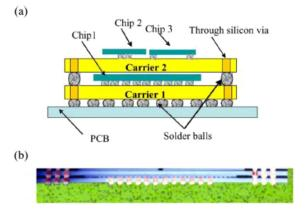
FIG. 64. (a) Schematic of 3D stack package and (b) cross section of 3D stack package.
