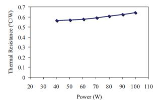
FIG. 76. Thermal resistance versus power input for the 3D package. <sup>108</sup> Reproduced with permission from Khan *et al.*, "3-D packaging with through-silicon via (TSV) for electrical and fluidic interconnections," IEEE Trans. Compon., Packag., Manuf. Technol. **3**(2), 221 (2013). Copyright 2013 Institute of Electrical and Electronics Engineers.
