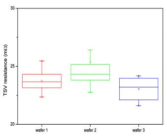
FIG. 42. Measurement results of TSV resistance.
