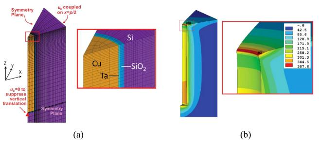
FIG. 82. Modeling of wafer cracking stress induced around a TSV. (a) Finite element model for the analysis and (b)  $\sigma_1$  (in MPa) induced in Si. <sup>124</sup> Reproduced with permission from Chan *et al.*, "Thermo-mechanical design rules for the fabrication of TSV interposers," IEEE Trans. Compon., Packag., Manuf. Technol. **3**(4), 633 (2013). Copyright 2013 Institute of Electrical and Electronics Engineers.
