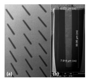
FIG. 16. X-ray (a) and X-SEM images (b) of  $10\,\mu\mathrm{m}\times100\,\mu\mathrm{m}$  TSV after ECP.
