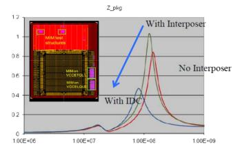
FIG. 49. Effect of decoupling capacitor for 2.5D IC power planes. <sup>101</sup> Reproduced with permission from Zhe *et al.*, "Development of an optimized power delivery system for 3D IC integration with TSV silicon interposer," in *Proceedings of IEEE Electronic Components and Technology Conference (ECTC)* (2012), pp. 678–682. Copyright 2012 Institute of Electrical and Electronics Engineers.
