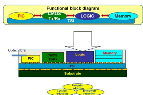
FIG. 7. Functional schematic of electronic–Photonic Integrated Circuits (PIC) on 2.5D TSI.
