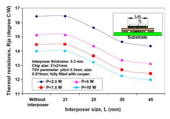
FIG. 61. Junction to ambient thermal resistance for different TSV interposer size. <sup>109</sup> Reproduced with permission from Hoe *et al.*, "Effect of TSV interposer on the thermal performance of FCBGA package," in 11th IEEE Electronics Packaging Technology Conference (EPTC) (2009). Copyright 2009 Institute of Electrical and Electronics Engineers.
