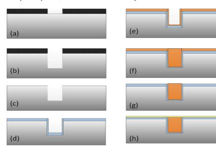
FIG. 8. Major process modules in TSV formation. (a) TSV mask lithography, (b) deep Si etch, (c) PRS and wafer cleaning, (d) liner oxide deposition, (e) barrier metal and Cu seed sputtering, (f) Cu ECP, (g) Cu CMP, and (h) TSV capping deposition if needed.
