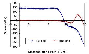
FIG. 90. Graph of stress (S33) along mid plane of bond for the full pad and the ring pad.<sup>132</sup> Reproduced with permission from Zhang *et al.*, "A low stress bond pad design for low temperature solder interconnections on through silicon vias (TSVs)," IEEE Trans. Compon., Packag., Manuf. Technol. **1**(4), 510 (2011). Copyright 2011 Institute of Electrical and Electronics Engineers.
