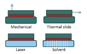
FIG. 32. Temporary bonding and debonding processes.
