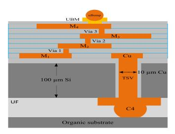
FIG. 40. Cross section view of through Si interposer.
