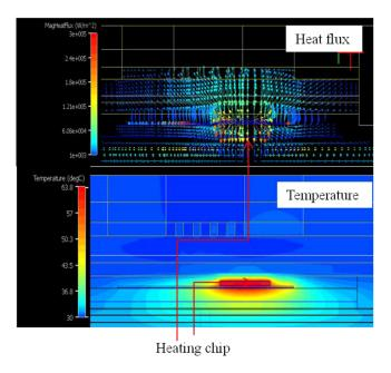
FIG. 78. Heat flux and temperature profiles for the molded package under cold plate cooling for determining the top thermal resistance.
