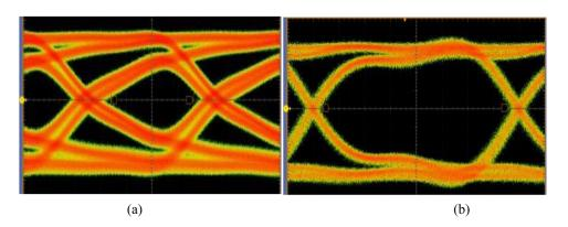
FIG. 46. Eye diagrams of 2 Gbps for 25 mm long (a) BEOL interconnect thickness 1  $\mu$ m, width 2  $\mu$ m, and pitch 4  $\mu$ m and (b) RDL interconnect thickness 3  $\mu$ m, width 3  $\mu$ m, and pitch 6  $\mu$ m.
