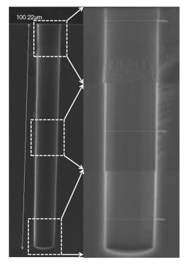
FIG. 10. TSV profile after deep reaction ion etching by using Bosch method. The size of TSV shown in the figure is 10  $\mu$ m in diameter and 100  $\mu$ m in depth, which has been widely accepted for interposer application.
