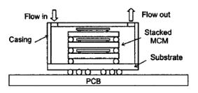
FIG. 70. Schematic of the direct cooling of 3D stacked MCM.
