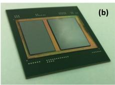
FIG. 37. (a) The top view of chip-onwafer and (b) chip-on-TSI-on-substrate.
