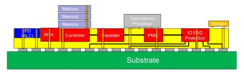
FIG. 106. Different design components on 2.5D active interposer—A schematic.
