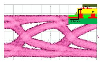
FIG. 48. Eye diagram of 25 Gbps for the off-TSI interconnect: M1-TSV-C4 bump.
