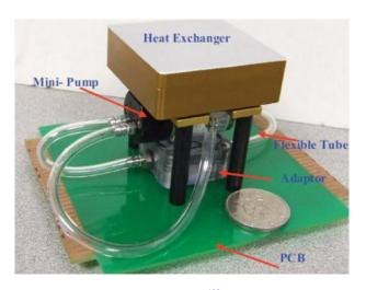
FIG. 75. Photograph of integrated cooling. <sup>108</sup> Reproduced with permission from Khan *et al.*, "3-D packaging with through-silicon via (TSV) for electrical and fluidic interconnections," IEEE Trans. Compon., Packag., Manuf. Technol. **3**(2), 221 (2013). Copyright 2013 Institute of Electrical and Electronics Engineers.
