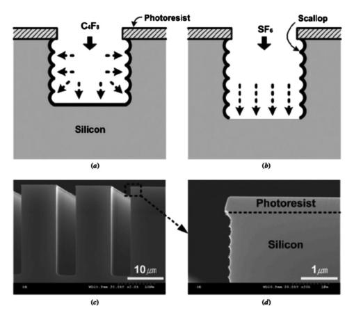
FIG. 9. Schematic of Bosch method: (a) sidewall passivation using C4F8, (b) Si isotropic etching using SF6, (c) SEM images of deep trenches, and (d) magnified SEM image of the sidewall showing nano-scallops.<sup>27</sup>
