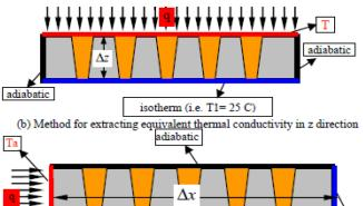
(c) Method for extracting equivalent thermal conductivity in x and y directions
