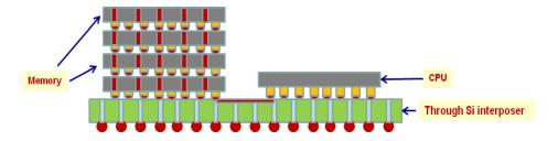
FIG. 5. Cross-section of CPU and 3D memory system showing the die level interconnections.
