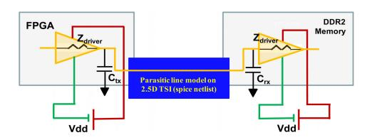
FIG. 99. Schematic to simulate the SI of a line in 2.5D TSI.
