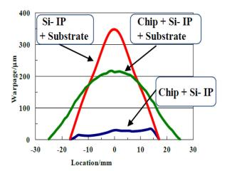
FIG. 39. Comparison of warpage after bonding. <sup>84</sup> Reproduced with permission from Murayama *et al.*, "Warpage control of silicon interposer for 2.5D package application," in *Proceedings of the IEEE-Electronic Components & Technology Conference* (ECTC) (2013), p. 879. Copyright 2013 Institute of Electrical and Electronics Engineers.
