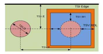
FIG. 93. Schematic illustrating the design rules for TSV.
