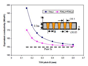
FIG. 55. Equivalent thermal conductivity of TSV interposer with different TSV pitches. <sup>109</sup> Reproduced with permission from Hoe *et al.*, "Effect of TSV interposer on the thermal performance of FCBGA package," in 11th IEEE Electronics Packaging Technology Conference (EPTC) (2009). Copyright 2009 Institute of Electrical and Electronics Engineers.
