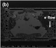
FIG. 27. SEM images of solder bump (a) without current stressing for 624 h and (b) with EM current stressing of  $6.4 \times 10^4 \text{A/cm}^2$  for 624 h at 150 °C.
