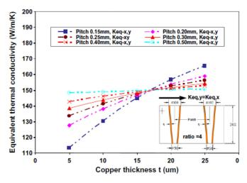
FIG. 58. Equivalent thermal conductivity Keq,x (=Keq,y) for partially filled TSV. <sup>109</sup> Reproduced with permission from Hoe *et al.*, "Effect of TSV interposer on the thermal performance of FCBGA package," in 11th IEEE Electronics Packaging Technology Conference (EPTC) (2009). Copyright 2009 Institute of Electrical and Electronics Engineers.
