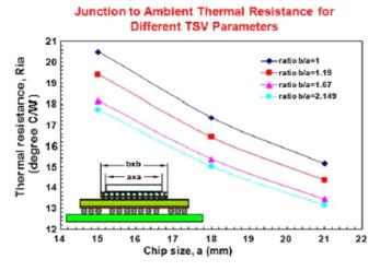
FIG. 63. Junction to ambient thermal resistance for different TSV sizes at different chip sizes. <sup>109</sup> Reproduced with permission from Hoe *et al.*, "Effect of TSV interposer on the thermal performance of FCBGA package," in 11th IEEE Electronics Packaging Technology Conference (EPTC) (2009). Copyright 2009 Institute of Electrical and Electronics Engineers.
