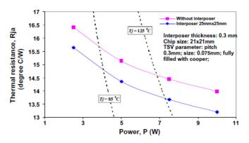
FIG. 60. Junction to ambient thermal resistance for different power dissipations. <sup>109</sup> Reproduced with permission from Hoe *et al.*, "Effect of TSV interposer on the thermal performance of FCBGA package," in 11th IEEE Electronics Packaging Technology Conference (EPTC) (2009). Copyright 2009 Institute of Electrical and Electronics Engineers.
