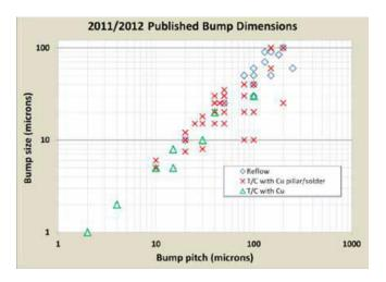
FIG. 105. Chip stacking bump sizes and pitches. <sup>146</sup> Reproduced with permission from Bersch *et al.*, "Cu-Cu direct bonding for ultra-high density chip-to-chip interconnects," in *Chip Scale Review Magazine*, Jul/Aug 2013, p. 20. Copyright 2013 Chip Scale Review.
