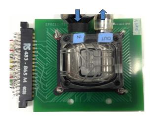
FIG. 77. Liquid cooling of 2.5D package with liquid cooling configuration.
