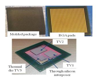
FIG. 67. The molded and bare die TSI package in  $26 \times 26$  BGA format. The Reproduced with permission from Zhang *et al.*, "Thermal characterization and simulation study of 2.5D packages with multi-chip module on through silicon interposer," in 15th IEEE Electronics Packaging Technology Conference (EPTC) (2013). Copyright 2013 Institute of Electrical and Electronics Engineers.
