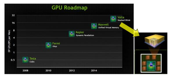
FIG. 103. Graphics processing unit (GPU) roadmap from Nvidia. <sup>141</sup> Reproduced with permission from *J.-H. Huang*, "Connecting people with ideas," paper presented at GPU Technology Conference, Nvidia, 2013. Copyright 2013 Nvidia Corporation.
