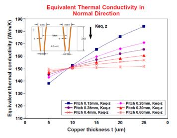
FIG. 57. Equivalent thermal conductivity Keq,z for partially filled TSV. <sup>109</sup> Reproduced with permission from Hoe *et al.*, "Effect of TSV interposer on the thermal performance of FCBGA package," in 11th IEEE Electronics Packaging Technology Conference (EPTC) (2009). Copyright 2009 Institute of Electrical and Electronics Engineers.
