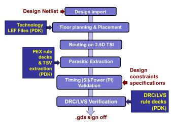
FIG. 96. 2.5D IC physical design flow.
