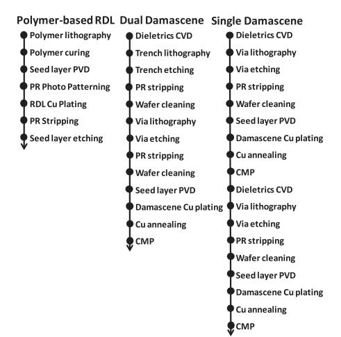
FIG. 18. Comparison of process steps of different Cu wiring processes, i.e., polymer-based RDL, dual damascene, and single damascene.
