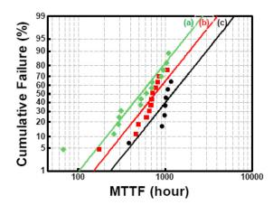
FIG. 28. Log-normal distribution of EM failure at 150 °C under various current densities of (a)  $6.4 \times 10^4 \,\text{A/cm}^2$ , (b)  $5.6 \times 10^4 \,\text{A/cm}^2$ , and (c)  $5.1 \times 10^4 \,\text{A/cm}^2$ .
