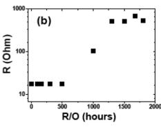
FIG. 25. Resistance as a function of storage time during HTS test at (a) 150 °C and (b) 180 °C.
