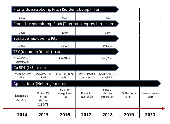
FIG. 104. Roadmap for different components of 2.5D TSI technology.
