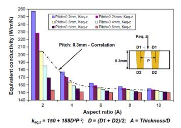
FIG. 53. Equivalent thermal conductivity in normal z-direction (keq,z). <sup>109</sup> Reproduced with permission from Hoe *et al.*, "Effect of TSV interposer on the thermal performance of FCBGA package," in 11th IEEE Electronics Packaging Technology Conference (EPTC) (2009). Copyright 2009 Institute of Electrical and Electronics Engineers.
