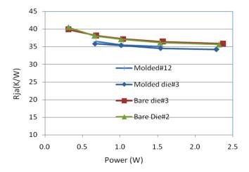
FIG. 68. Measured Theta JA test jig under natural convection condition for both molded and bare die package. <sup>112</sup> Reproduced with permission from Zhang *et al.*, "Thermal characterization and simulation study of 2.5D packages with multi-chip module on through silicon interposer," in 15th IEEE Electronics Packaging Technology Conference (EPTC) (2013). Copyright 2013 Institute of Electrical and Electronics Engineers.
