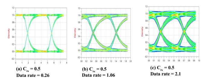
FIG. 100. Eye diagram simulations for various data rates and driver impedances (0.26 GT/s–2.1 GT/s). (a)  $C_{tx}=0.5$  data rate = 0.26, (b)  $C_{tx}=0.5$  data rate = 1.06, and (c)  $C_{tx}=0.5$  data rate = 2.1.
