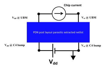
FIG. 101. Schematic for static IR Drop analysis.
