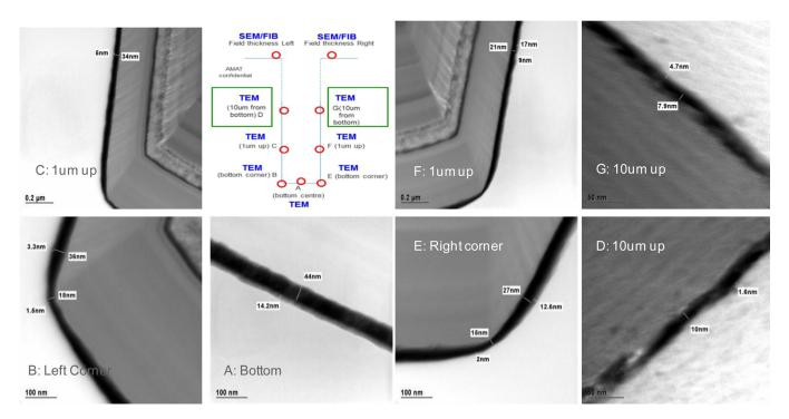
FIG. 14. SEM images of Ti and Cu as barrier and seed layer for  $10 \, \mu m \times 100 \, \mu m$  TSV.
