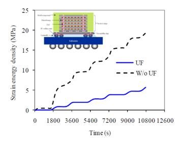
FIG. 88. Effect of underfill on C4 bumps of a 3D package. [31] Reproduced with permission from Che *et al.*, "The study of thermo-mechanical reliability for multi-layer stacked chip module with through-silicon-via (TSV)," in *Proceedings of 12th Electronics Packaging Technology Conference (EPTC)*, Singapore, December 2010, p. 743. Copyright 2012 Institute of Electrical and Electronics Engineers.
