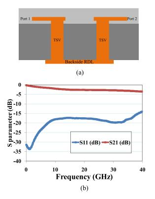
FIG. 47. (a) DUT and (b) S parameter characterization of TSV-back side RDL-TSV interconnect.
