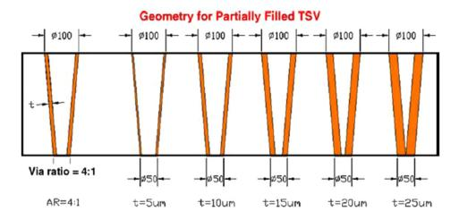
FIG. 56. Geometry for partially filled TSV.<sup>109</sup> Reproduced with permission from Hoe *et al.*, "Effect of TSV interposer on the thermal performance of FCBGA package," in 11th IEEE Electronics Packaging Technology Conference (EPTC) (2009). Copyright 2009 Institute of Electrical and Electronics Engineers.
