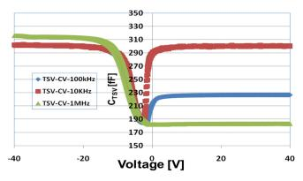
FIG. 43. Measured TSV capacitance result with different bias voltage and frequency.
