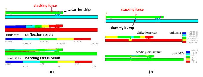
FIG. 86. Die deflection  $u_y$  and bending stress  $u_x$  results during a chip stacking process for (a) original bump layout design and (b) optimized bump layout design. Perpoduced with permission from Che *et al.*, "Structure design optimization and reliability analysis on a pyramidal-shape three-die-stacked package with through-silicon via," IEEE Trans. Device Mater. Reliab. **12**(2), (2012). Copyright 2012 Institute of Electrical and Electronics Engineers.
