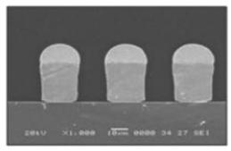
FIG. 21. SEM images of Cu pillar bumps.
