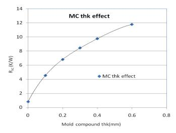
FIG. 79. Effect of molding compound thickness on the Rjc.
