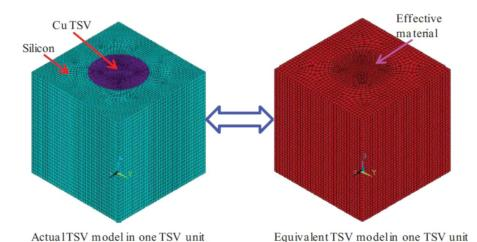
FIG. 85. Use of an effective material to develop an equivalent TSV model. <sup>128</sup> Reproduced with permission from Che *et al.*, "Development of wafer-level warpage and stress modeling methodology and its application in process optimization for TSV wafers," IEEE Trans. Compon., Packag., Manuf. Technol. **2**(6), 944 (2012). Copyright 2012 Institute of Electrical and Electronics Engineers.
