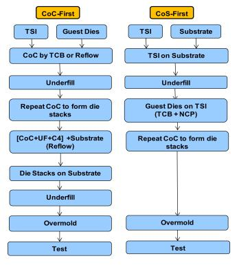
FIG. 34. Assembly flow options for TSI packaging.
