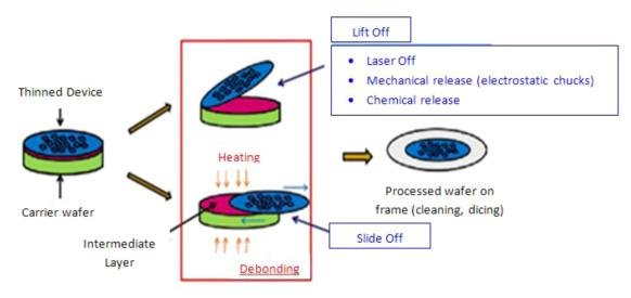
FIG. 31. A typical debonding process flow.
