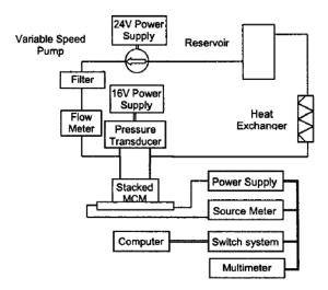
FIG. 71. Schematic of liquid cooling characterization.
