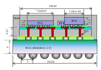
FIG. 66. The schematic of the multi chip module on through Si interposer, with TV1 behind TV3. The SEM image of TSV under thermal chip bumps is also shown. (Unit: mm). 112 Reproduced with permission from Zhang *et al.*, "Thermal characterization and simulation study of 2.5D packages with multi-chip module on through silicon interposer," in 15th IEEE Electronics Packaging Technology Conference (EPTC) (2013). Copyright 2013 Institute of Electrical and Electronics Engineers.
