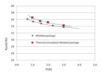
FIG. 69. Comparison of averaged simulation results versus measurements for the junction to ambient thermal resistances under natural convection condition. <sup>112</sup> Reproduced with permission from Zhang *et al.*, "Thermal characterization and simulation study of 2.5D packages with multi-chip module on through silicon interposer," in 15th IEEE Electronics Packaging Technology Conference (EPTC) (2013). Copyright 2013 Institute of Electrical and Electronics Engineers.
