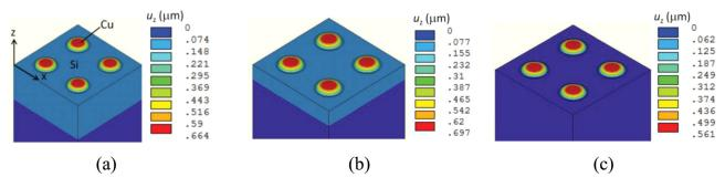
FIG. 83. Copper protrusion FEM results: (a) Right after ramping up to 400 °C, (b) held for 30 min at 400 °C, and (c) cooled down to room temperature. Peproduced with permission from Che *et al.*, "Study on Cu protrusion of through-silicon via," IEEE Trans. Compon., Packag., Manuf. Technol. **3**(5), 732 (2013). Copyright 2013 Institute of Electrical and Electronics Engineers.
