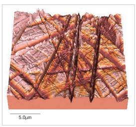
Figure 2.6: AFM topographical scan of a glass surface. The micro and nano-scale features of the glass can be observed, showing the roughness of the material; from: http://en.wikipedia.org/wiki/ File:AFMimageRoughGlass20x20.JPG [Accessed 10 August 2012].
