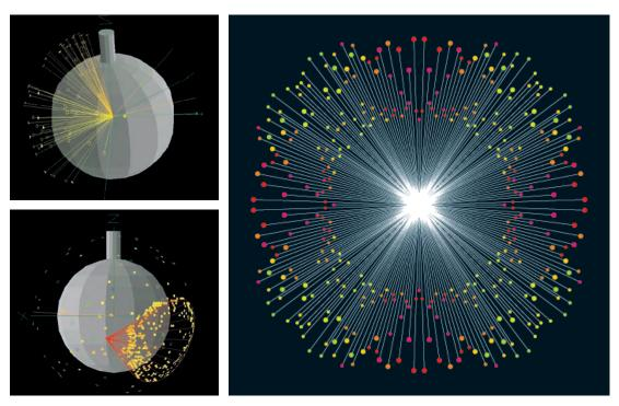
Figure 3.22 (top left): When a neutrino strikes the heavy water of the Sudbury Neutrino Observatory (SNO) detector, a faint cone of light spreads out from that point to SNO's light sensors which surround the spherical vessel of heavy water. In this neutrino event, 75 of the 9600 light sensors observed a photon of light. The lines indicate the direction from the neutrino strike to the sensors, from http://www.sno.phy.queensu.ca/event/event.html [Accessed 10 July 2011].
