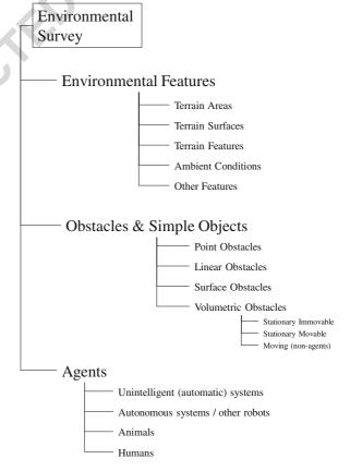
Fig. 4 Classification scheme used in environmental survey hazard analysis
