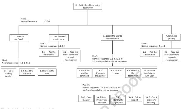
Fig. 6 Guide robot hierarchical task diagram
