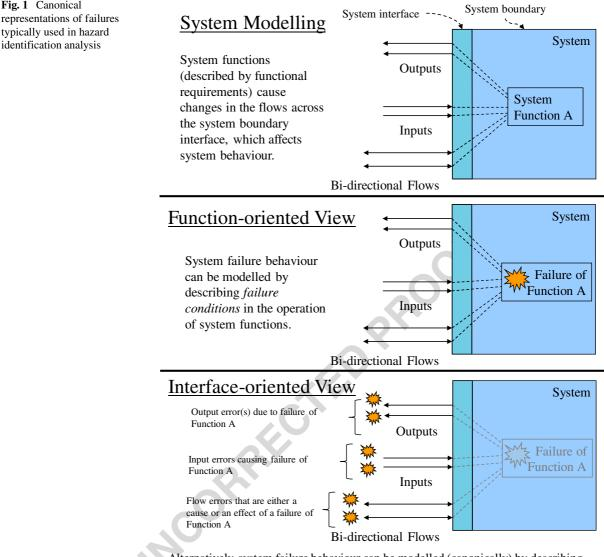
Alternatively, system failure behaviour can be modelled (canonically) by describing *boundary flow errors* that cause or arise from failures of internal system functions.
