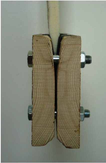
Figure 14. Side view of tapered wooden grip holding foam test piece. Abrasive paper can be seen on the tapered edges. Each half of wooden grip was 18.5mm thick, from which the scale can be judged.
