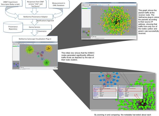
By zooming in and comparing the metadata harvested about each sender, we can see that it's the difference in configuration of OTG2 that is resulting in different throughput results.
