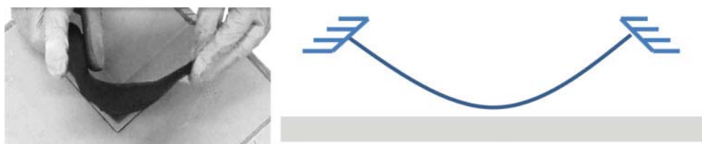
Figure 6 (Left) 'Two-handed guiding' used to both position and shape a ply during Task 4. (Right) Schematic force diagram of technique (not to scale)
