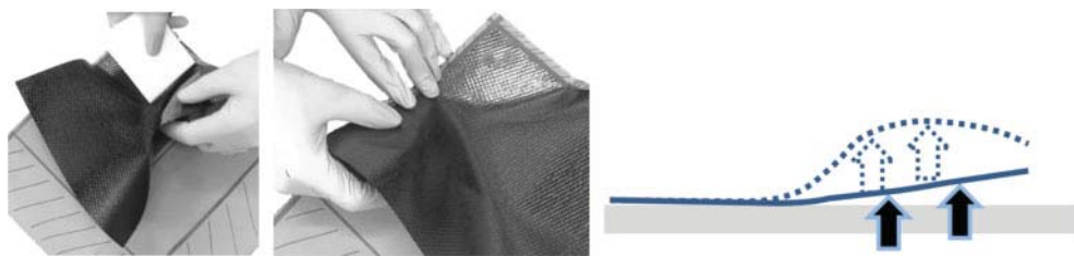
Figure 12 Example of folding material to accommodate the shear during task 8 (not to scale)
