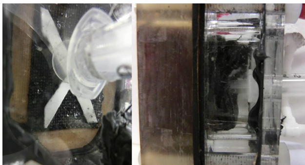
Fig. 2. Catholyte formation in situ as droplets on both the 2D (left) and folded 3D (right) electrodes; catholyte droplets are more visible on the 2D surface.
