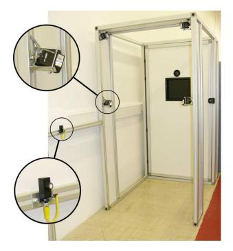
Figure 2.5 The Photoface capture device. One of the light sources and the ultrasound trigger are shown in the enlarged areas (Zafeiriou et al., 2013).
