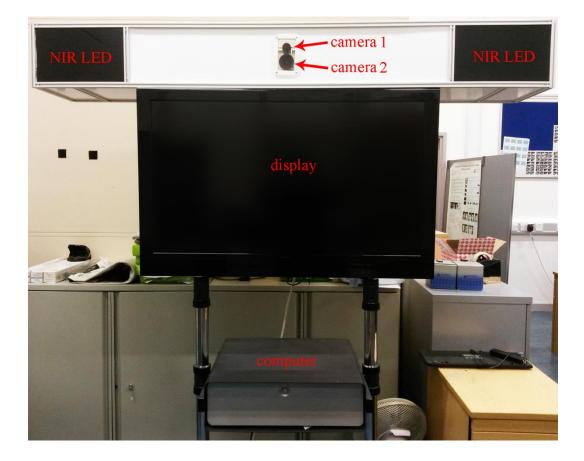
Figure 3.1 System structure for the 2D+3D imaging system
