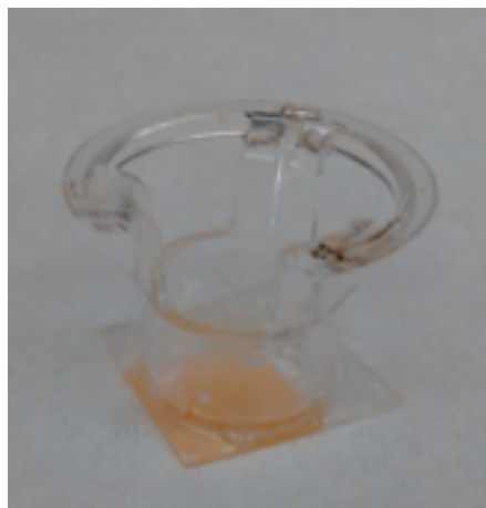
Fig. 2 Completed Transwell array glued with PDMS to a quarter of the original array.
