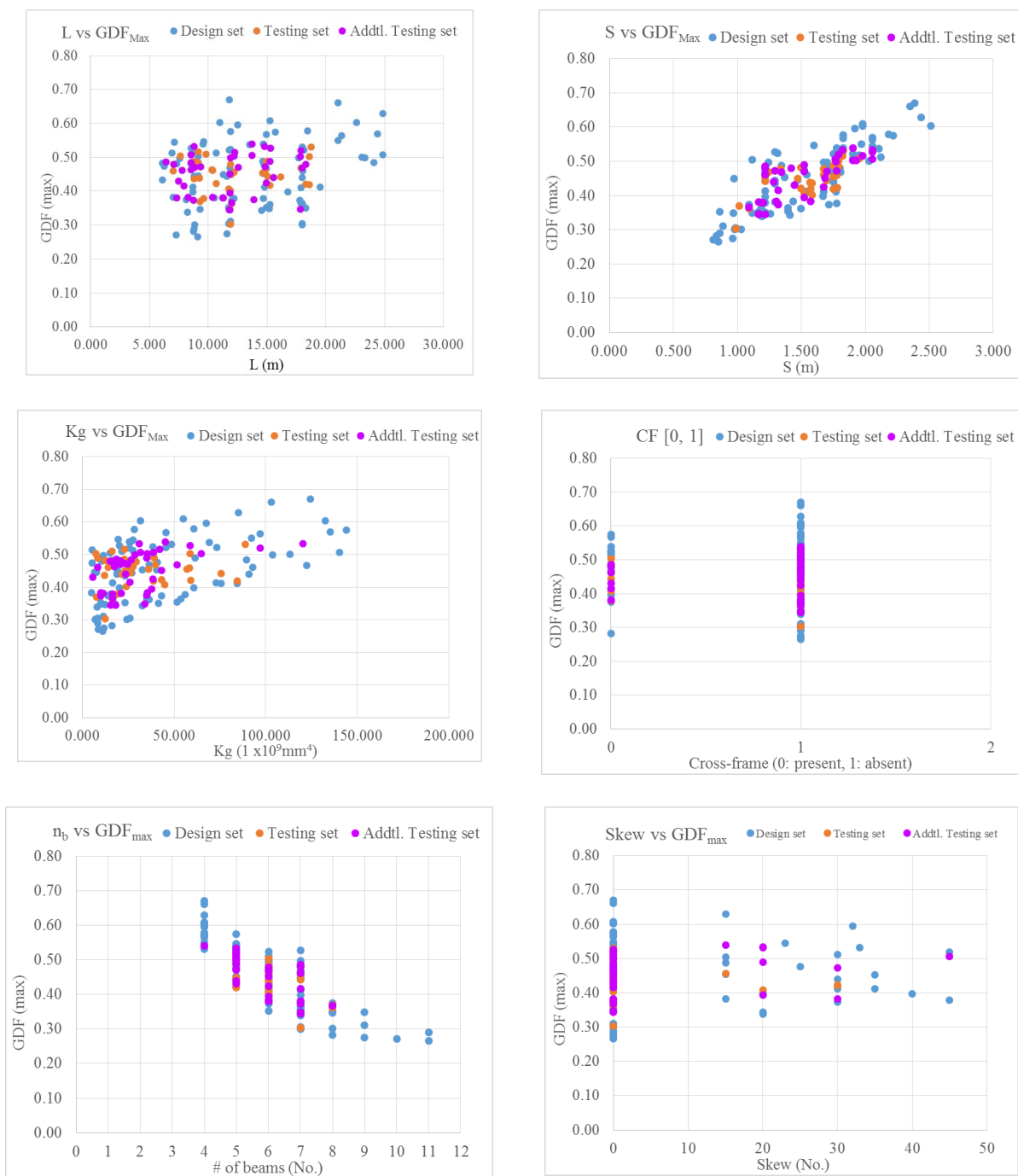
Figure 42. Moment GDFs vs. Governing Parameters for 90 Bridges in Design Set
