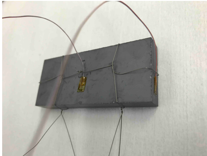
Figure 1: Silicon sample used in this experiment. The sample has not a mirror finishing surface. T-type thermocouples and the Ti-6Al-4V wires are shown.
