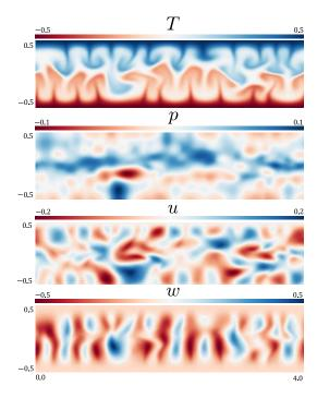
Figure 2: An illustration of a typical solution to the Rayleigh–Bénard problem (Eqns. (3a)-(3c)). The contours respectively show the solution for temperature (T), pressure (p), and the two velocity components (u and w). For this simulation case Pr=1,  $Ra=10^6$ , and  $L_x=4L_z=4$  [m]. The spatial resolution is  $n_x=4\times n_z=512$ , and upon an adaptive time stepping scheme the presented solution above is obtained at t=25 [s].
