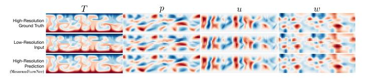
Figure 6: Sample tuples of low-resolution input data for MeshfreeFlowNet, the high-resolution super-resolved data by MeshfreeFlowNet, and the ground truth high-resolution data for the 4 physical parameters of the Rayleigh-Bénard problem, i.e., T, p, u, w as the temperature, pressure, and the x and z components of the velocity. The contours correspond to the MeshfreeFlowNet model evaluation presented in Table 4 for  $Ra = 1 \times 10^8$ .
