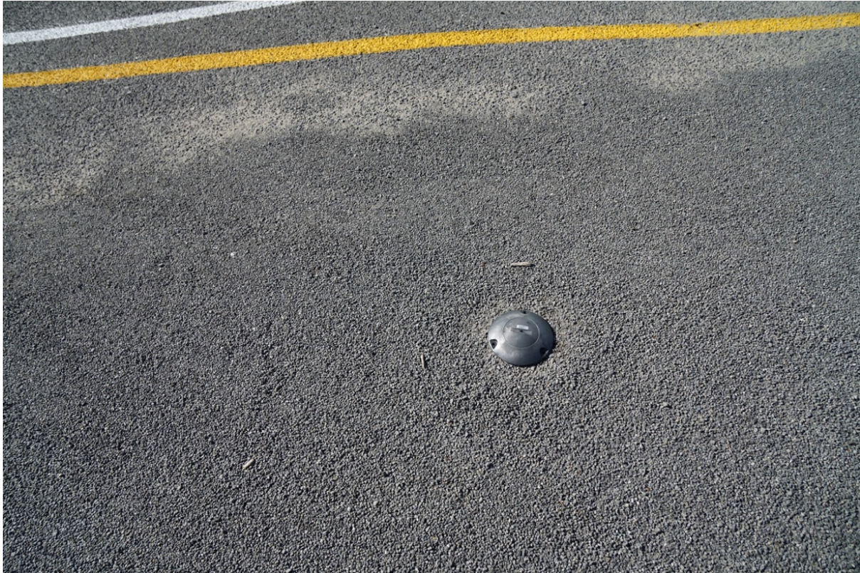
Figure 5.7: A Campermate sensor installed at the Akaroa boat launch freedom camping area. Source: Author
