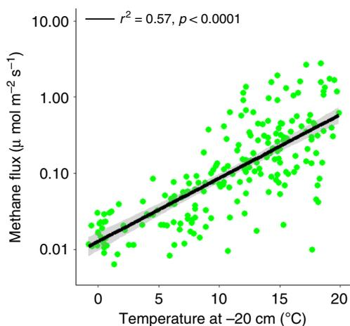
**Fig. 3 Methane flux from S1 Bog.** Exponential temperature response of surface  $\text{CH}_4$  emissions following five years of warming. Measurements were made 6–8 times per year during 2015–2018. Linear regressions with 95% confidence intervals are shown in black and gray, respectively. Note the log-scale on the y-axis.
