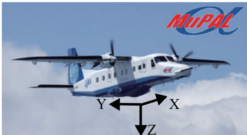
Fig. 6.2 MuPAL- \alpha (©JAXA) and its body-fixed coordinate system. X: out the nose of the aircraft. Y: out the right wing. Z: down through the bottom.
