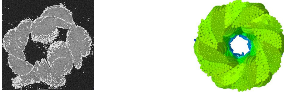
Figure 9: Comparison of the braid cross-sections. a) CT scan cross-section image. b) Braid model cross-section.
