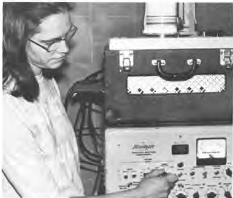
Fig. 1. Student helper operating Fourier Wave Analyzer. Permanent spectra are etched into the graphite coated paper on top of the instrument.
