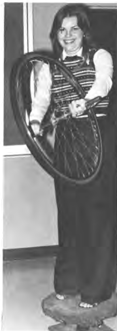
Fig. 4. Bicycle wheel on rotating table with student demonstrator. The rotating table is made from a cast-off axle.
