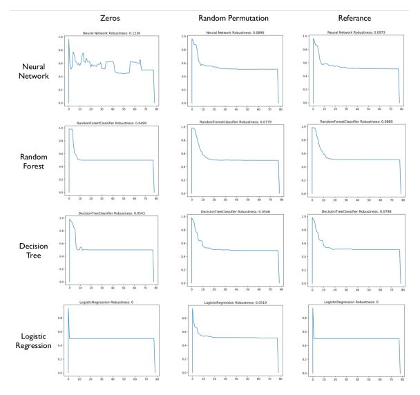
Fig. 6.3.1: Robustness plots with balanced accuracy on the y-axis and number of features deactivated on the x-axis
