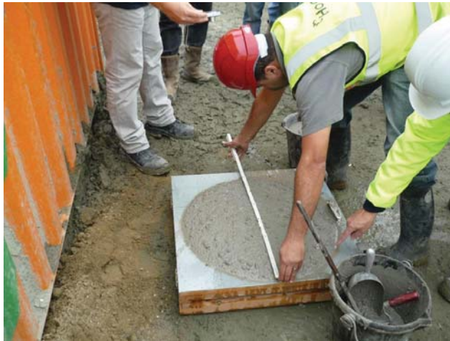
Figure 3: Flow measurement on fresh concrete at construction site
