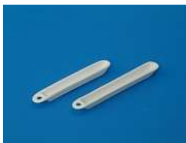
Figure 1.20 – The "shuttle" crucibles
