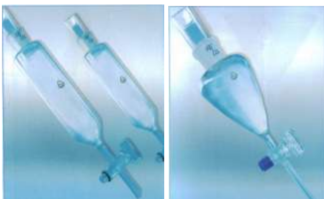
Figure 1.12 – separation (a) and drop (b) funnels
