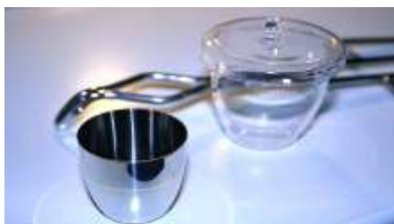
Figure 1.19 – Platinum and Quartz crucible
