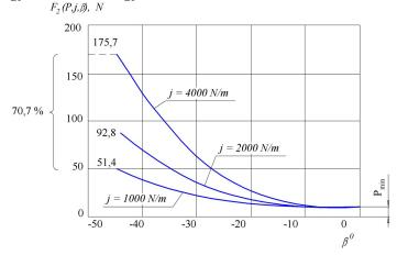
Fig. 4. Change of pedipulator driving force on the second stage of movement  $\beta = -45^0...0$  depending on the stiffness of the elastic elements using same values of the constants (see Fig. 3) and initial compression of the elastic element  $P = P_{min} = 10 N$
