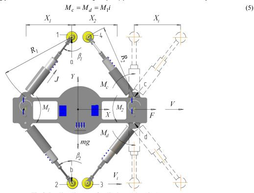
**Fig. 2. Loading diagram of pedipulator (plan view):** grippers 1, 2 – attached to the surface and 3, 4 – free from engagement with the surface, respectively
