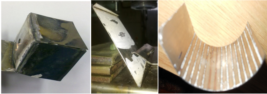
Fig. 4. Specimens formed by laser heat
