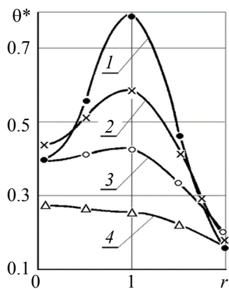
Fig. 2. The change in temperature \theta^* of tool along the radius at \varphi = 0 , z = -0.5 , \varphi_1 = \pi/3 , a^* = 1.0 , Pe = 4.5 for different values of r_0 : 1 – r_0 = 0.5 ; 2 – 0.75; 3 – 1.0; 4 – 1.5
