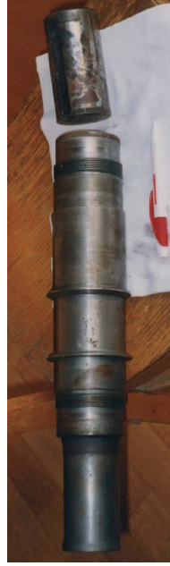
Fig. 14. Stepped drive broken shaft
