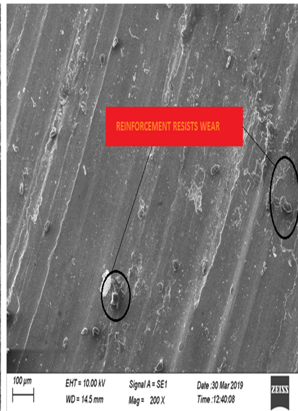
Fig. 8.b Worn surface of AL7075-12%TiB 2 -4.5%MoS 2
