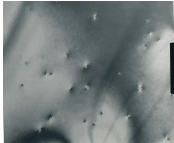
Figure 2. Defective structure of the sample after etching in the dark-field image. The mark in the photo corresponds to 250 nm.
