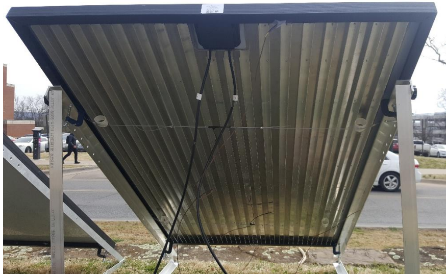
Figure 14. In-House Constructed Fins
