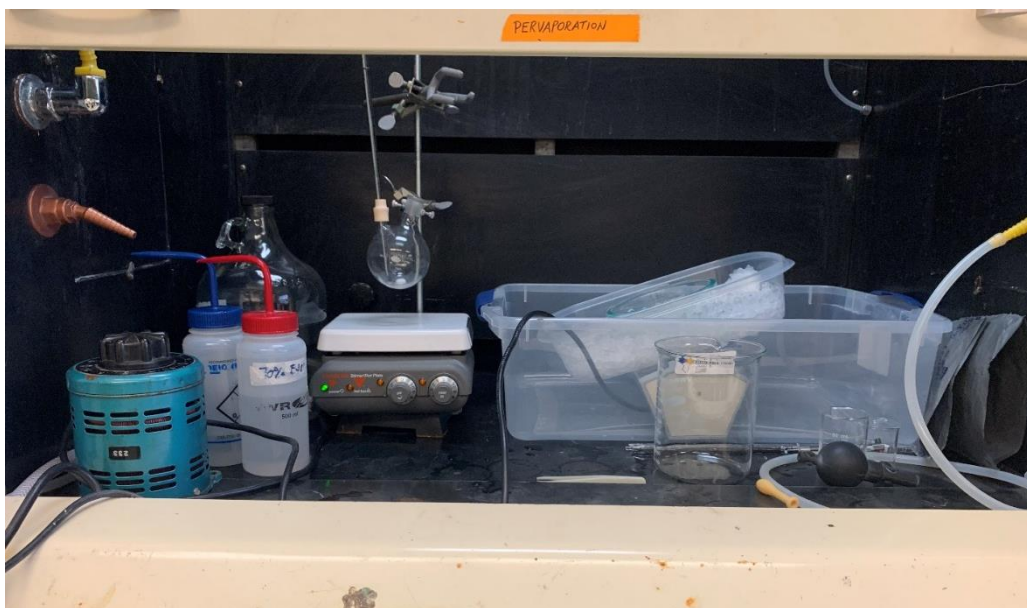
Figure 4 - Picture of experimental setup. Variable motor is glossy teal object on left, waste container in back left, two-neck flask with stirrer towards center left above hot plate, and mechanical rocker with three layers of containment on right.
