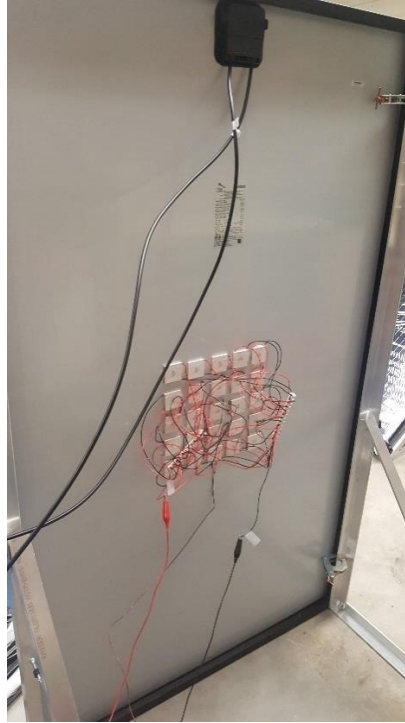
Figure 12. 25 TEGs on the back of a 300 W panel
