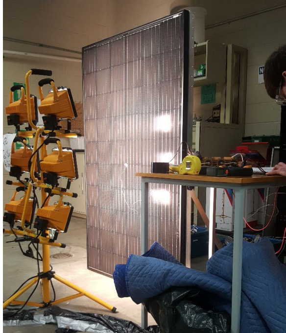
Figure 13. Indoor Testing Module
