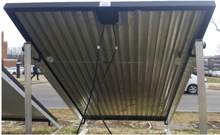
Figure 14. In-House Constructed Fins
