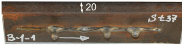
FIG. 1. Gravity drop-out of the melt in a full penetration welding of 20 mm thick S235JR steel plate using 13.9 kW laser power (YLR 20000 IPG) without weld pool support, the welding velocity was 0.5 \text{ m min}^{-1} .
