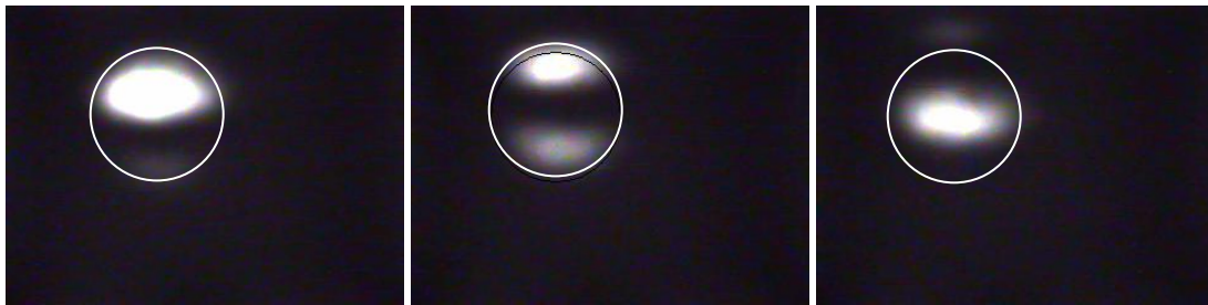
Figure 13: IR Interferogram of the moderate soot deposited chip with wavelength tuning.
