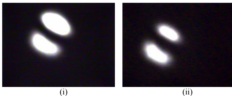
Figure 18: IR interferograms of the chip placed at 1100 °C for (i) 30 minutes and (ii) 2 hours.
