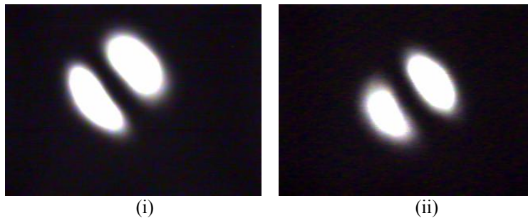
Figure 17: IR interferograms of the chip placed in the acid for (i) 1 hour and (ii) 24 hours.
