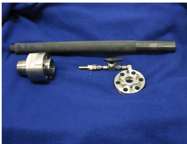
Fig.7. SiC temperature probe shown in an unassembled fashion.
