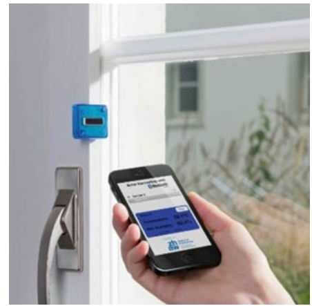
Fig.2 Sensor powered using energy harvesting
