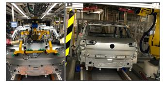
FIGURE 2. Fixture for the tailgate assembly process (left) and the Perceptron measurement station downstream (right).
