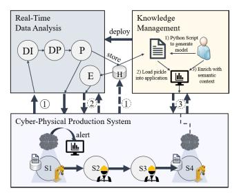
**FIGURE 9.** Possible deployment architecture based on the IDARTS framework [6]. Legend: DI - Data Ingestion; DP - Data Preprocessing; P - Prediction; E- Evaluation; H - Historical database; 1 - Prediction request; 1 (dashed) - Store ground truth; 2 (dashed) - Request mode evaluation; 3 (dashed) - Request updated model.
