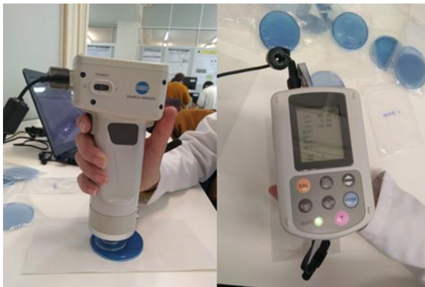
Figure 8 CHROMA METER CR-400 from Konica Minolta used to measure the color of films.
