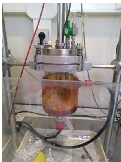
Figure 4 Reactor designed by the LSRE-LCM group for the synthesis of aqueous polyurethane dispersion.
