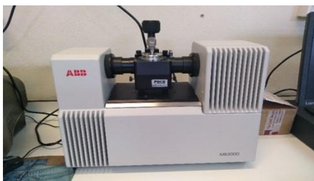
Figure 9 Fourier Transform Infrared (FTIR) equipment used to the analyze the films chemical structure
