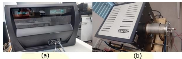
Fig. 2 - Main devices employed. (a) hotdisk equipment e (b) furnace.
