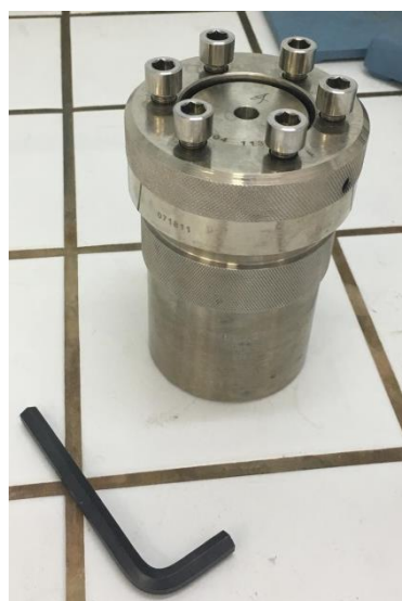
Figure 11. Reactor used to digestion of the sample.
