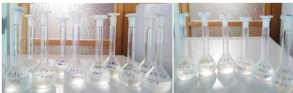
Figure 12. Samples after digestion, ready to be read on atomic absorption equipment.
