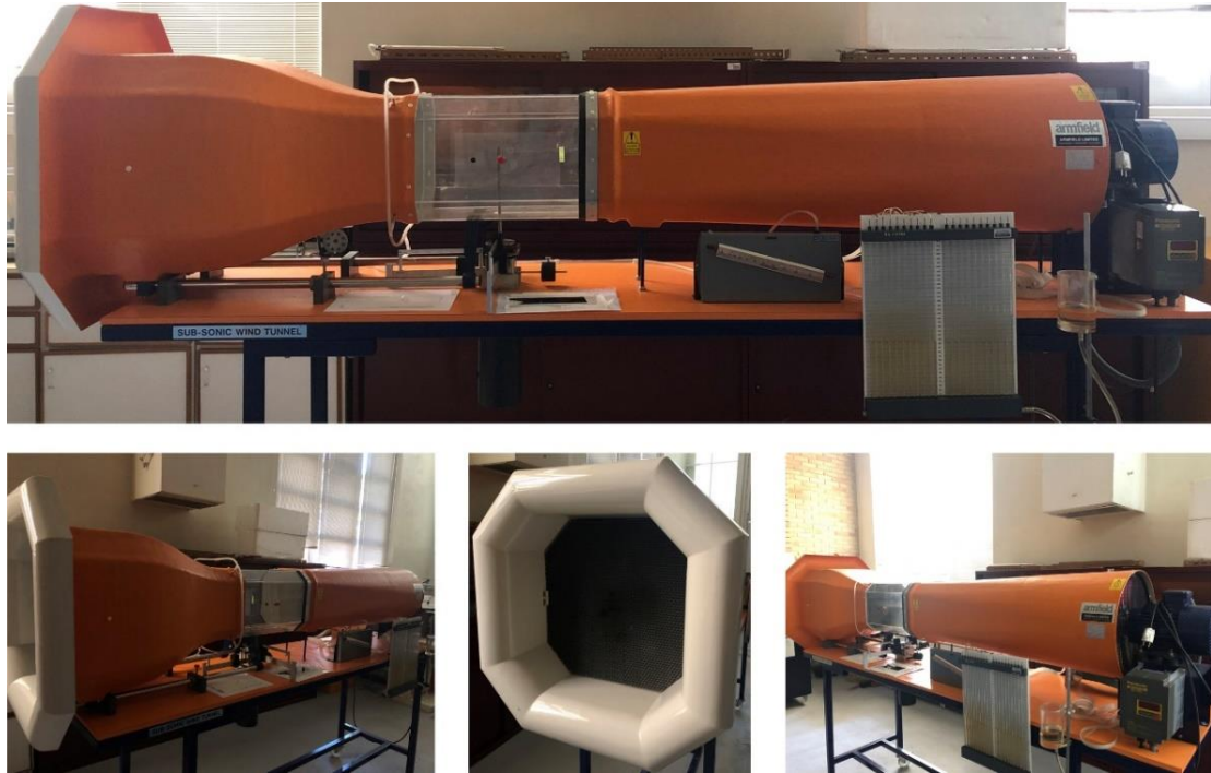
Figure 4.2 – Subsonic open-circuit suction type wind tunnel of LHMf from IPB.
