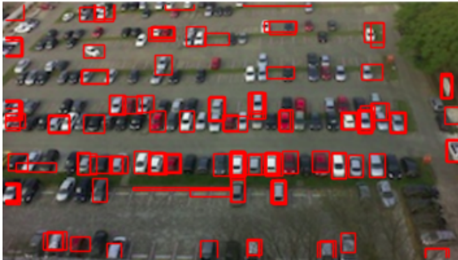
Figure 3.7: Corner Detection and bounding box drawing process.
