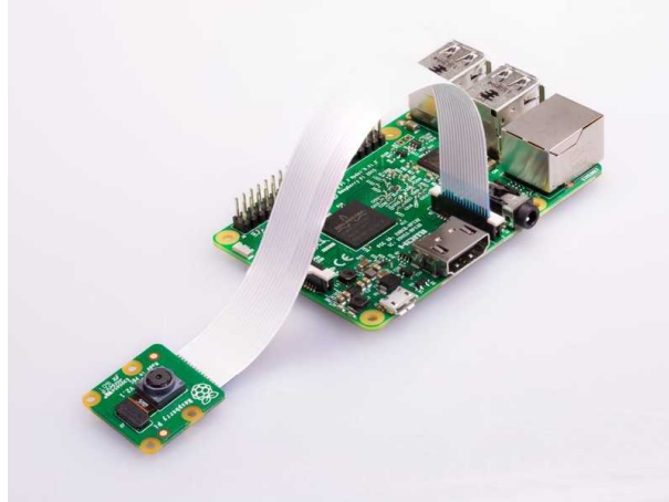
Figure 3.1: Raspberry Pi's structure integrated with RaspCam, reproduced from [54].
