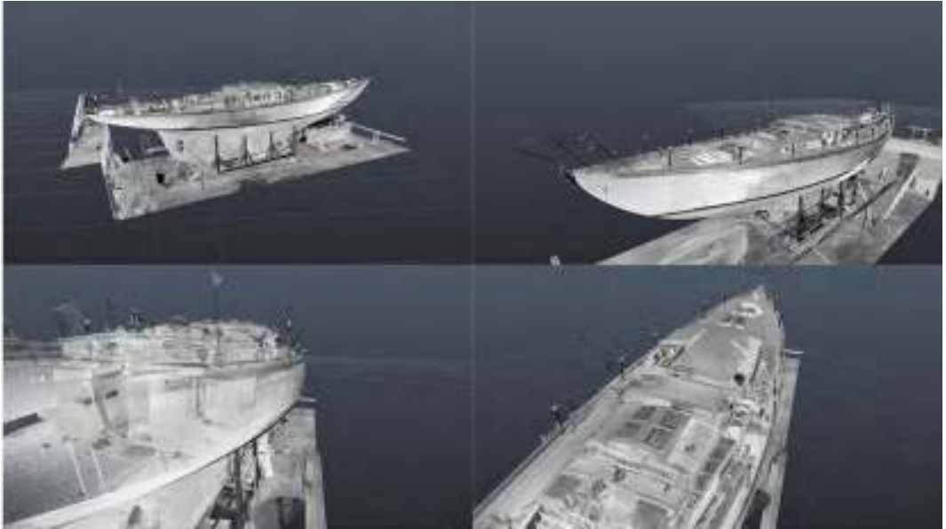
Fig. 5 Returning survey with laser scanner for optimal data acquisition for the restitution of the deck plan.
