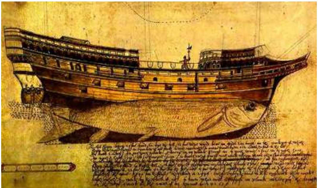
Fig. 4 The hull of a vessel inspired by the shape of a cod head and a mackerel tail. Matthew Baker, Fragment of Early English Shipwrightry (1586), Magdalene College, Pepys Library, Cambridge (Ms 2820, sheet n.d.).
