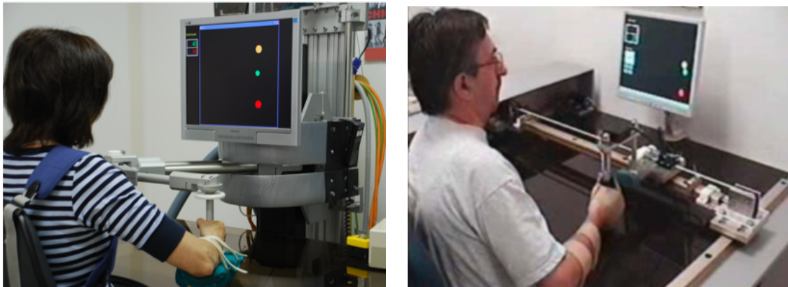
Figure 7.2 Experimental setup. Participants performed planar movements with the devices ‘Braccio di Ferro’ (BdF, left) (Casadio et al., 2006) or the MEchatronic system for MOfotor recovery after Stroke (MEMOS, right) (Colombo et al., 2005) (in-house prototype).
