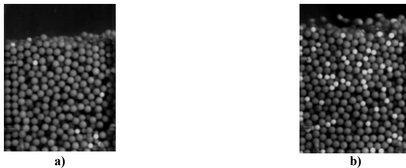
Figure 4 Experimental results (after 15 s) - Representative particle distribution in the bed at a superficial-velocity of 2.3 m/s (a) and 2.8 m/s (b)
