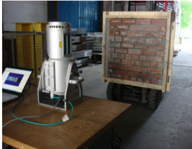
Figure 3: The scanning process of model sample 1 at the measuring distance of approximately 2m using the RIEGL LMS-Z420i
